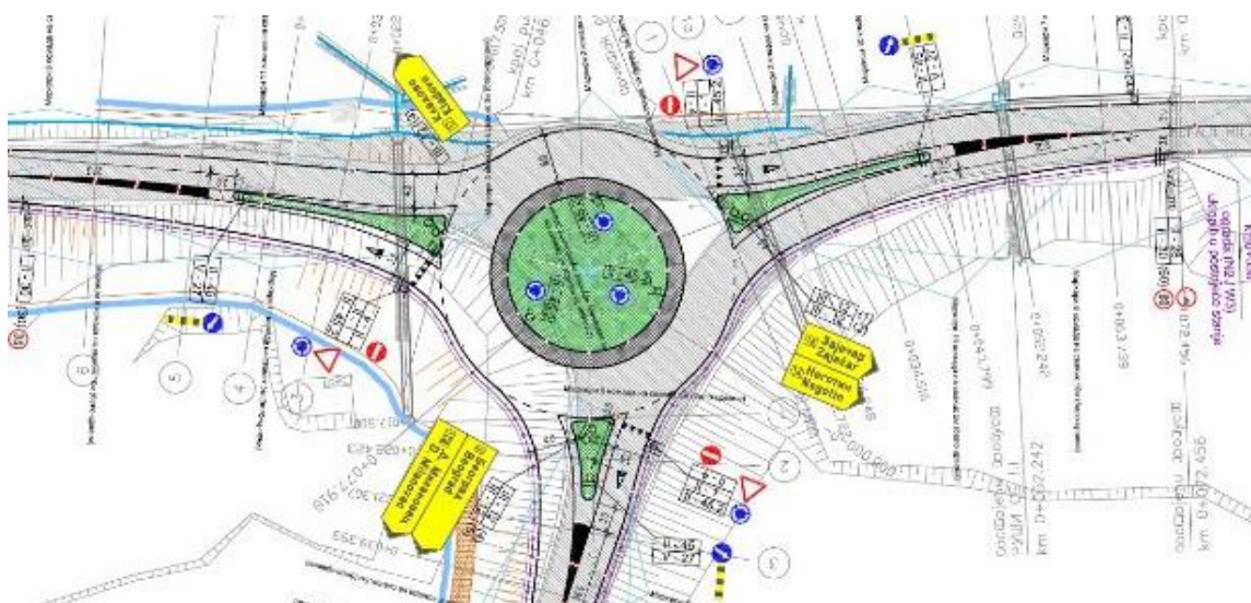
Example of traffic flows channelisation on approaches to the roundabout
